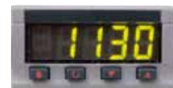
Over-temperature limit controller
