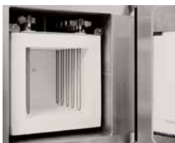
Molybdenumdisilicide heater and fiber insulation
