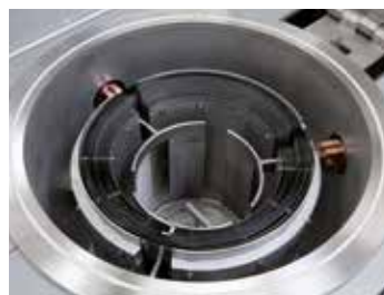
Cylindrical retort with tungsten heating
