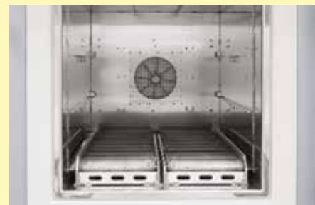
Roller conveyor in furnace chamber
