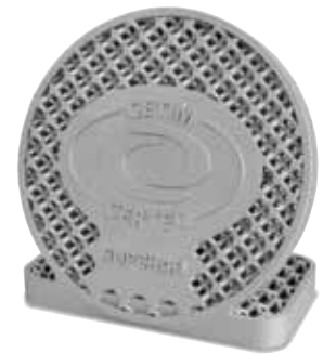
Printed aluminum part, heat treated in model N 250/85 HA (Manufacturer CETIM CERTEC on SUPCHAD platform)
