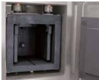
Graphite heating chamber
