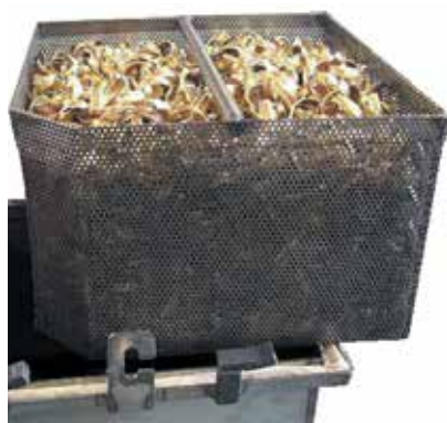
Charging basket for top charging
