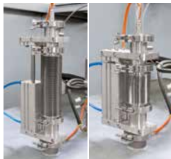
Thermocouple, type S with automatic pull-out device for precise control results in the low temperature range
