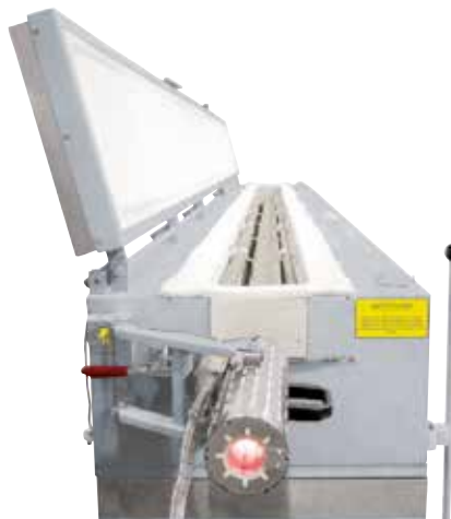
Strand annealing furnaces based on a tube furnace with a length of 6 meters
