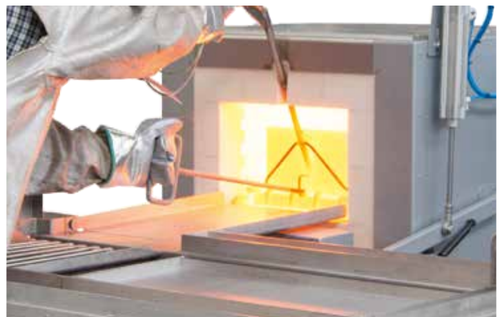
Protective gas hardening system with furnace N 41/H
