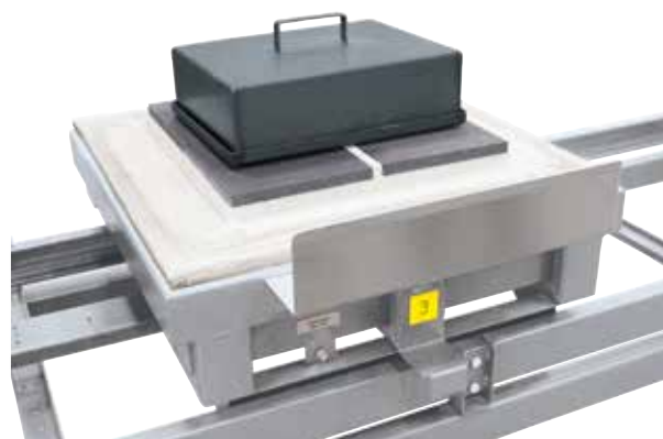
Protective gas box for similar furnace
