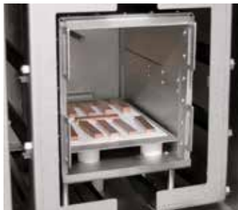
Heat treatment of copper bars under hydrogen in retort furnace VHT 8/16-MO
