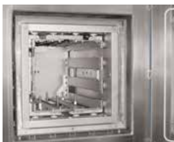
Molybdenum or tungsten heating chamber
