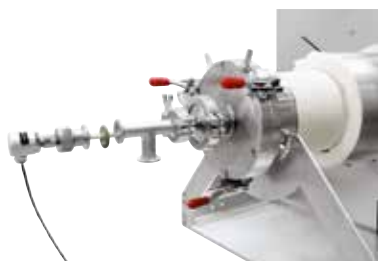
Thermocouple for charge control in the furnace RHTH 120/600/18
