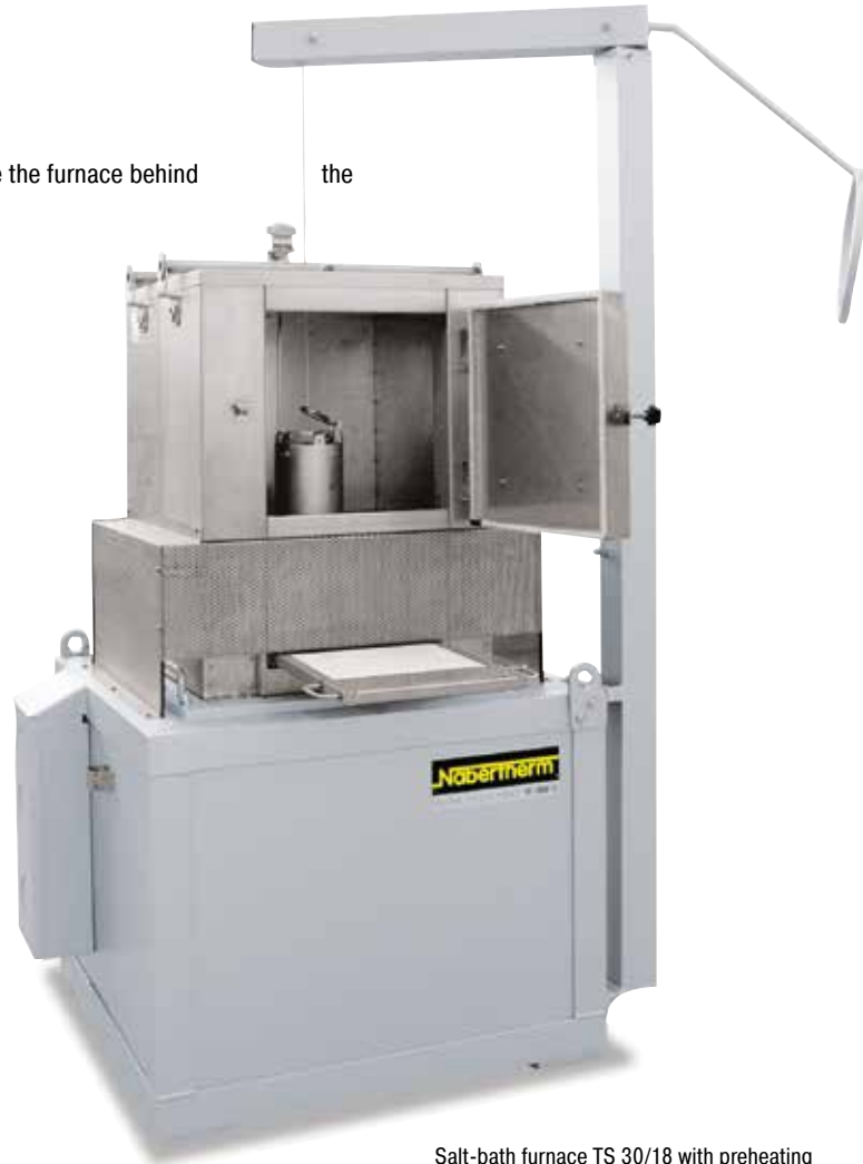
Salt-bath furnace TS 30/18 with preheating chamber above the salt bath and charging aid for immersion of the charge
