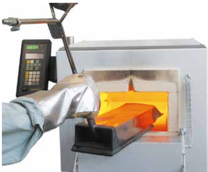
Hardening in annealing tray with alloy bag
