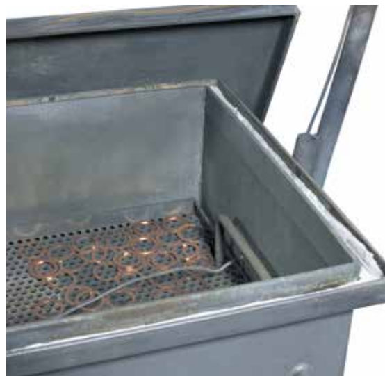
Heat treatment under protective gas atmosphere in a protective gas box incl. charge thermocouple
