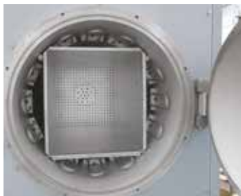
Inside heating in retort furnace NRA ../06
