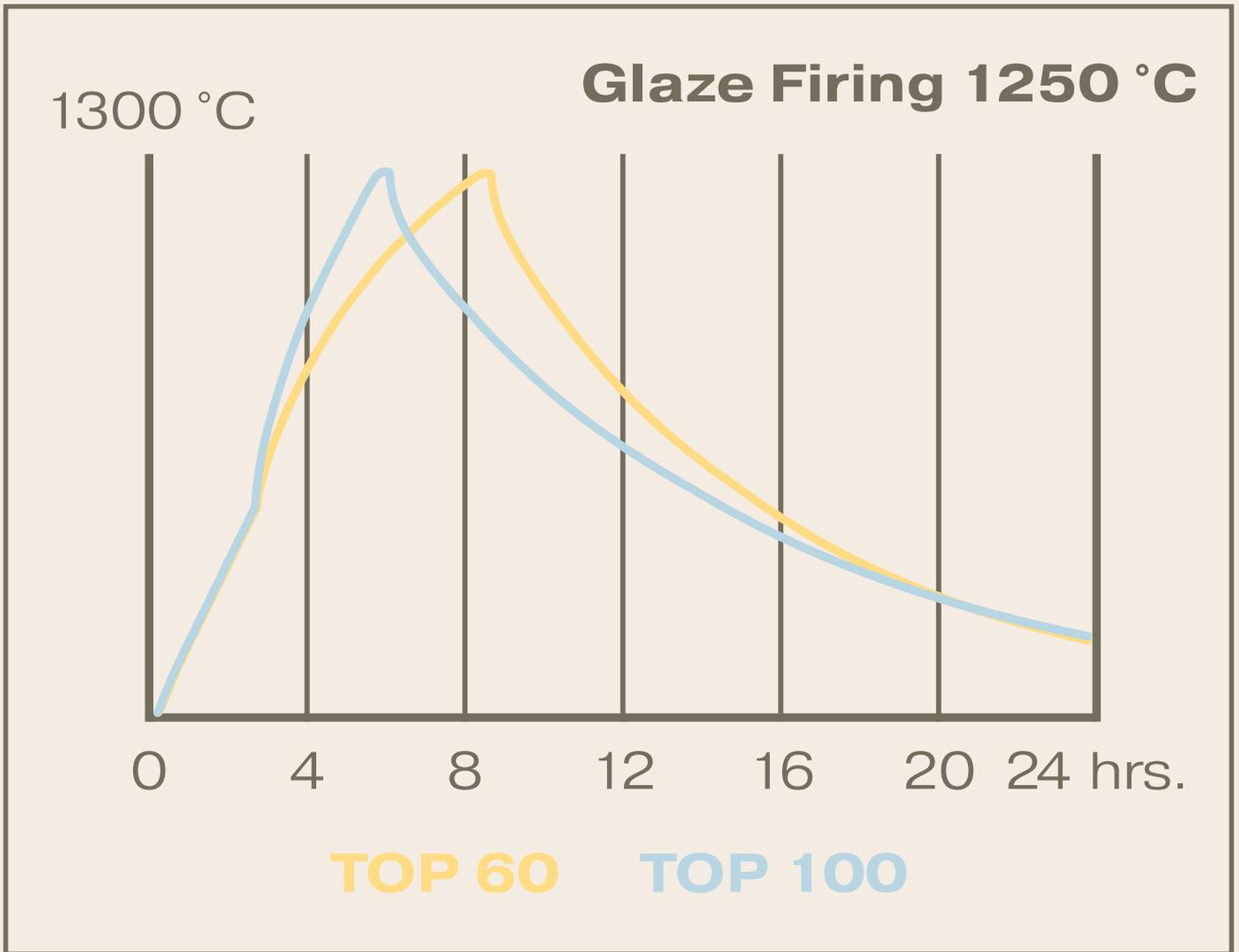
Example curve of a glaze firing
