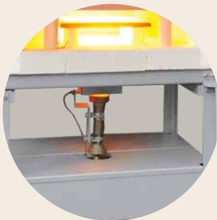
15 kW propane gas mounted under the kiln
