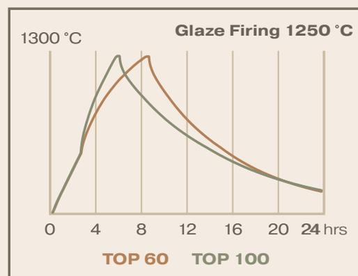
\*Bisque firing 950 °C, glaze firing 1250 °C. Charge weight incl. kiln furniture: Top 60 - 18 kg, Top 100 - 30 kg. Calculated energy price: 0,30 €/kWh.
