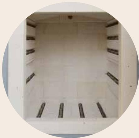
Three-sided heating with elements protected in grooves
