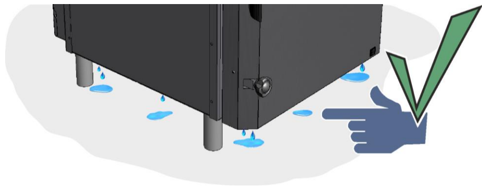
Fig. 67: Condensation accumulations during the first firings (similar to picture)
