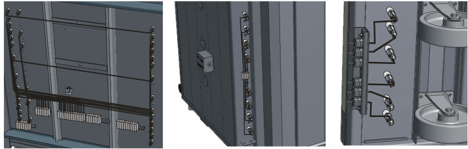
Example: Heating element terminals on back wall (floor)
