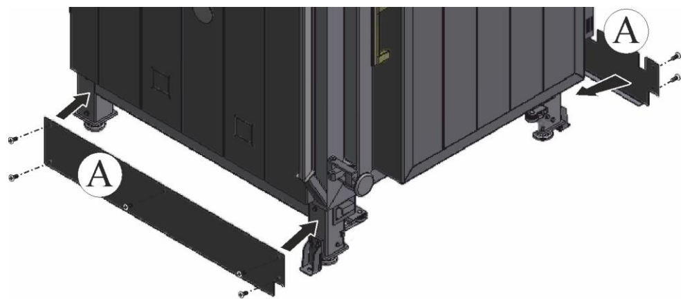
Fig. 46: Assembling the side panels (similar to figure)
