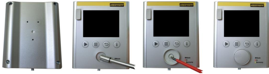
Fig. 16: Installing the controller circuit board - part 3 (similar to picture)
