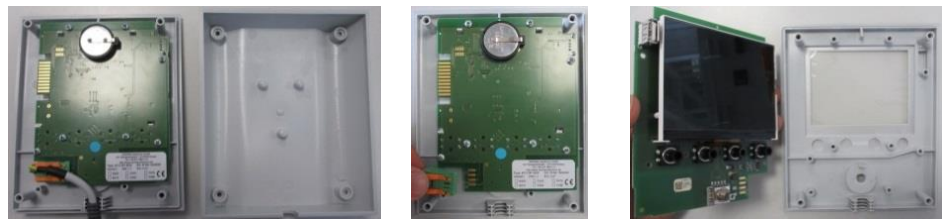
Fig. 13: Removing the controller circuit board - part 2 (similar to picture)
