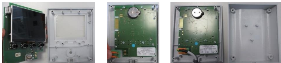
Fig. 15: Installing the controller circuit board - part 2 (similar to picture)
