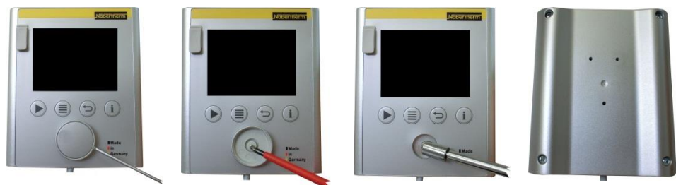
Fig. 12: Removing the controller circuit board - part 1 (similar to picture)
